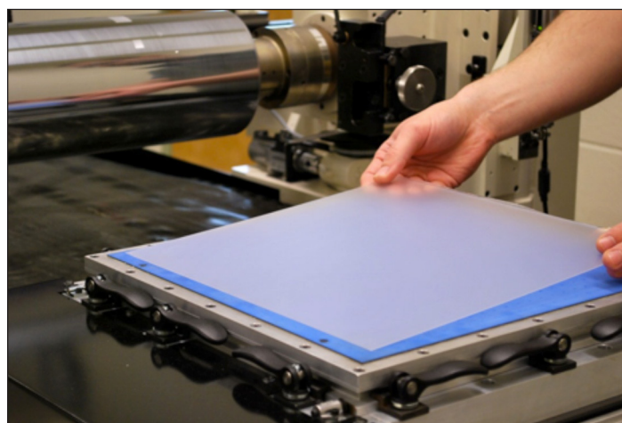
Figure 1. Loading of rigid substrate onto platen of precision sheetfed rotogravure press, which can be run with or without glove box enclosure in place. (Reproduced courtesy of Erika Rebrosova, Center for the Advancement of Printed Electronics.)
