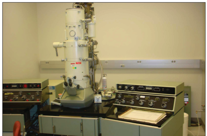
Figure 4. Electron microscope on a vibration isolation slab in Building 62.
