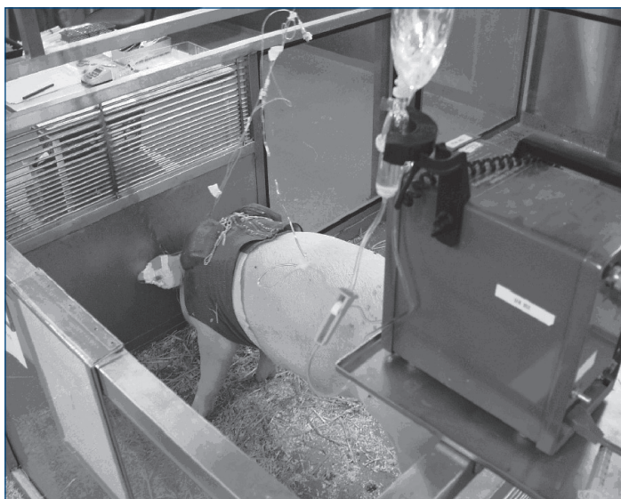
Figure 2. The pig is a good model for evaluating the performance and biocompatibility of implantable glucose sensors due to practical, anatomical (e.g., subcutis), physiological, and immunological reasons. Here seven sensors were implanted in the subcutis, and performance of the sensors was tested with a setup of a glucose pump connected to a venous (implanted in the jugular vein) catheter and a catheter for blood sampling. After termination of the experiment, tissue around sensors were sampled (see Figure 3).
