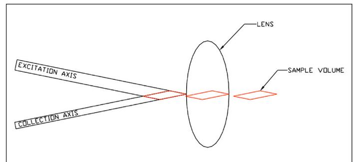
**Figure 2.** Diagram of volume of measurement.
