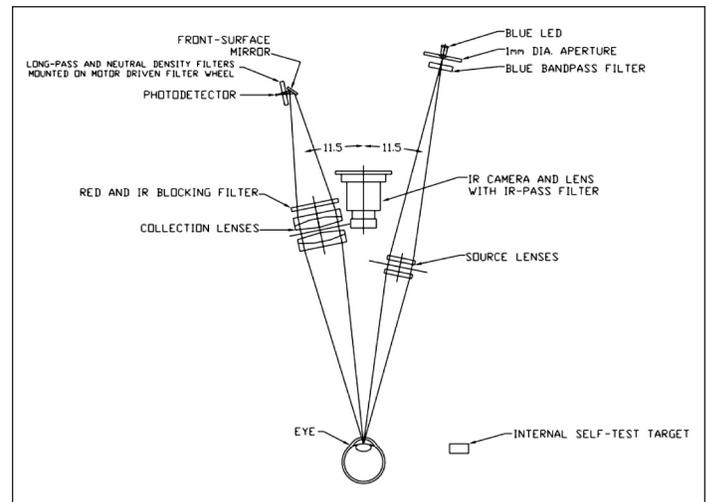
**Figure 1.** Optical system. Dia, diameter.
