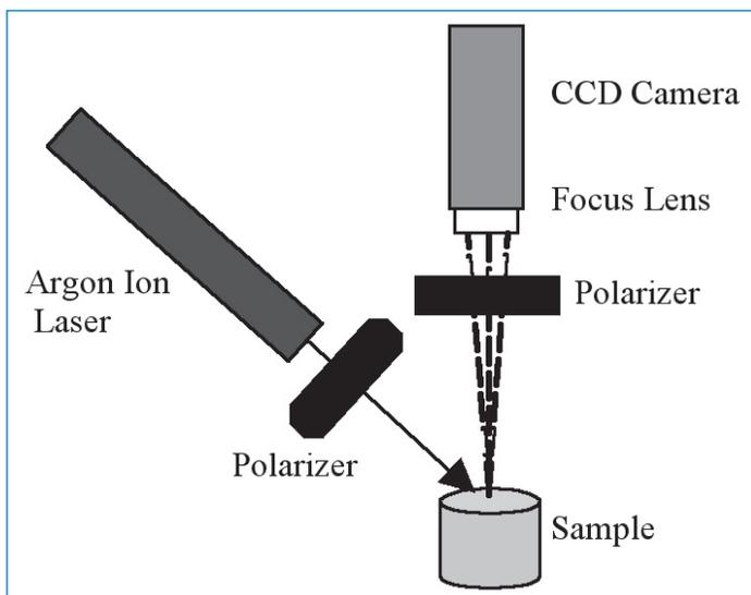
**Figure 1.** Experimental setup for the polarization imaging system.
