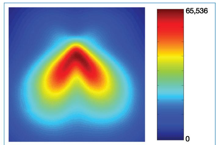
**Figure 2.** Raw image obtained for a glucose level of 50 mg/dl with a pseudo-color map applied. The color bar represents respective levels of light intensity.
