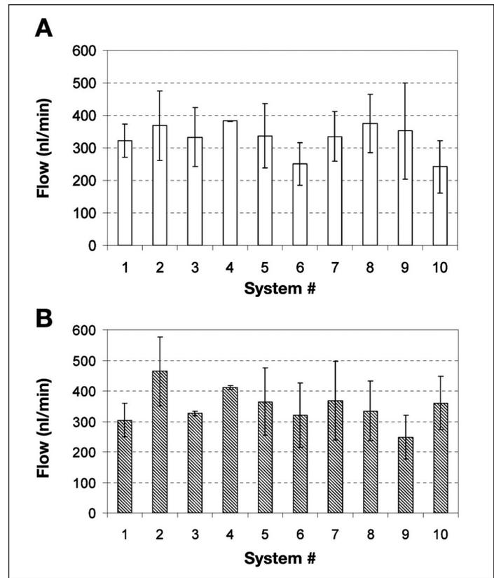
**Figure 3.** Variation of the mean flow rate of 10 different CRT systems calculated from recorded CRT flow rate sensor measurements over a total monitoring time of 120 h (A) *in vitro* and (B) *in vivo*.
