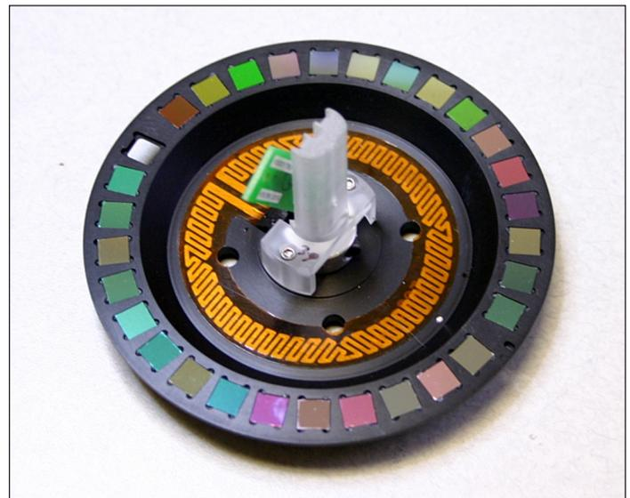
**Figure 3.** Fixed-filter wheel with 25 unique wavelength filters, used in the custom spectrometer.
