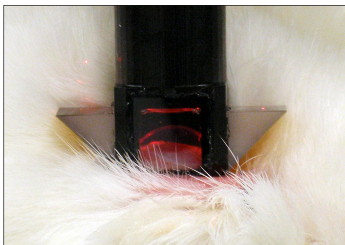
Figure 3. The coupling of the glucose-sensing optical signal through the aqueous humor of a NZW rabbit.
