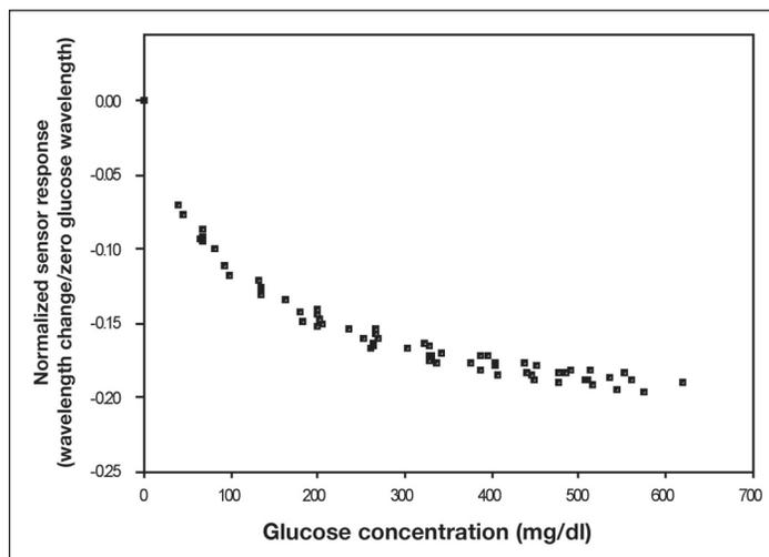
**Figure 3.** Normalized glucose in PBS calibration plots at pH 7.40 and 37°C for different slices of 3 mol% MBA, 12 mol% 3-APB, and 12 mol% ATMA holograms made on 4 different days and derived from three different hydrogel batches. Calibration data were normalized by dividing the diffraction peak shift at each concentration by the starting wavelength.
