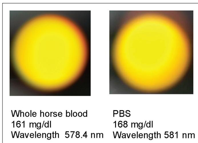
**Figure 1.** The color of a 3 mol% MBA, 12 mol% 3-APB, and 12 mol% ATMA hologram in whole (horse) blood and PBS at pH 7.40 and 37°C. The glucose concentrations of the samples were adjusted to be approximately the same so that they replay the same color (yellow).
