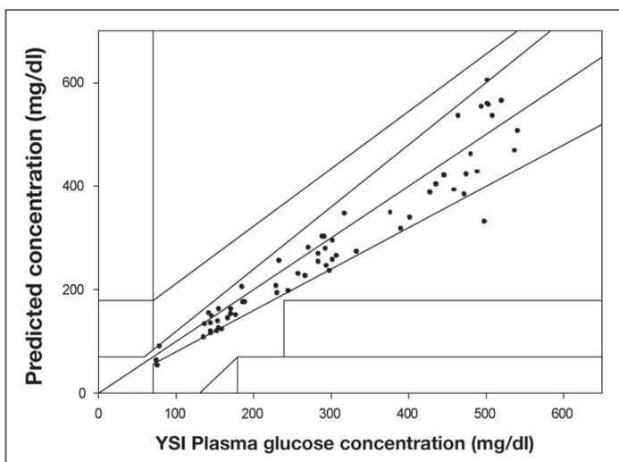
**Figure 4.** The measurement of glucose in human plasma samples containing different types of endogenous and exogenous substances using a 3 mol% MBA, 12 mol% 3-APB, and 12 mol% ATMA hologram at pH 7.40 and 37°C. Results are plotted against the true values obtained using the YSI reference method. Test levels of the substances are specified in Table 1.
