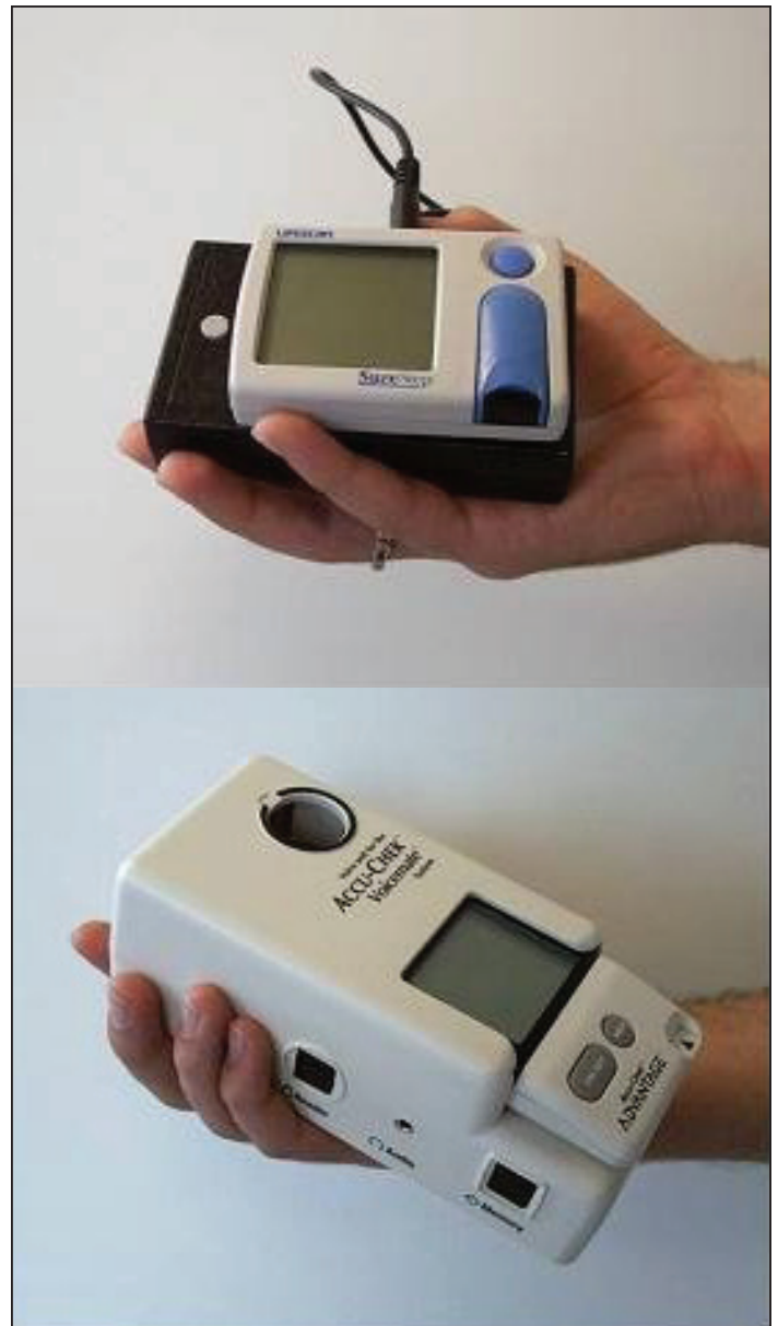
Figure 1. In 2003, accessibility to BGM technology was provided by the Mini-Digi voice module ( top , with the LifeScan SureStep) and the Accu-Chek Voicemate ( bottom , with the Accu-Chek Advantage).
