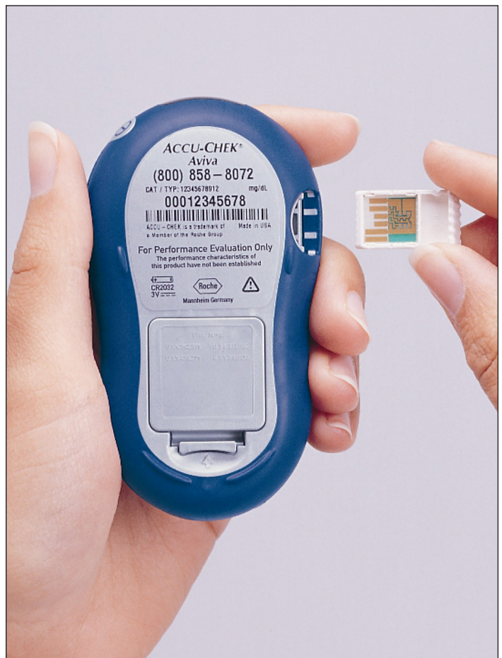
Figure 2. An electronic code chip for Roche's ACCU-CHEK® Aviva glucose meter. The chip contains batch-specific code information.
