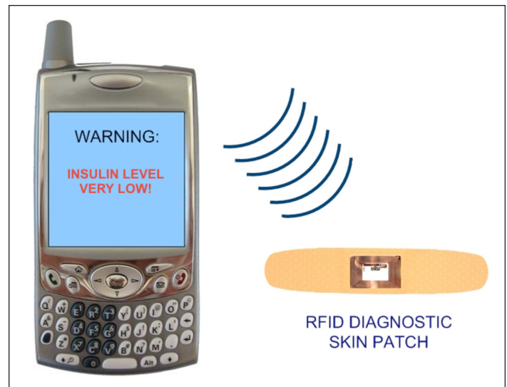
Figure 1. Intermediate phase with “patch” communicating only to mobile device. Illustration courtesy of Gentag, used with permission.
