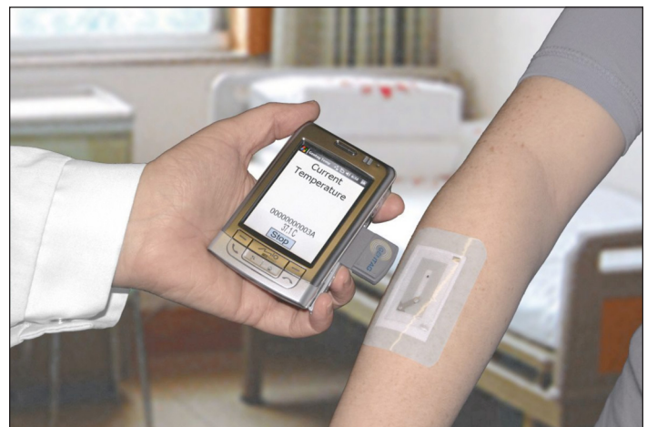
Figure 2. Temperature sensor being read by a specially equipped mobile device with an add-on RFID interrogator (right side of device). Illustration courtesy of Gentag, used with permission.
